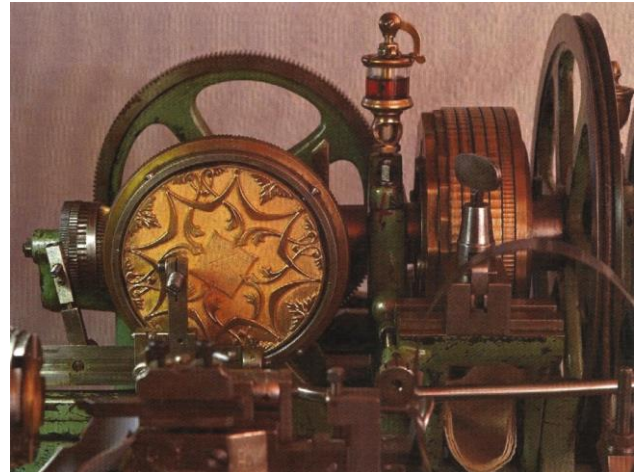
"Machine à tapisserie", which reproduces a pattern from a model.
